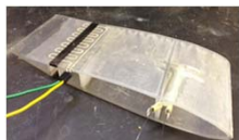
Printed wing with embedded actuator and printed strain gage
