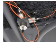
212 high sensitivity accelerometers
