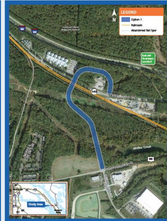
Two-lane divided facility with a reduced design speed (140 - foot Limit of Disturbance)
