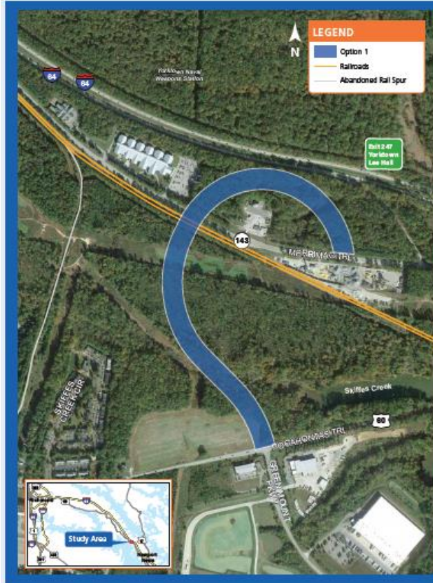
Four-lane divided freeway facility that was anticipated to tie into other projects (225 - foot Limit of Disturbance)
