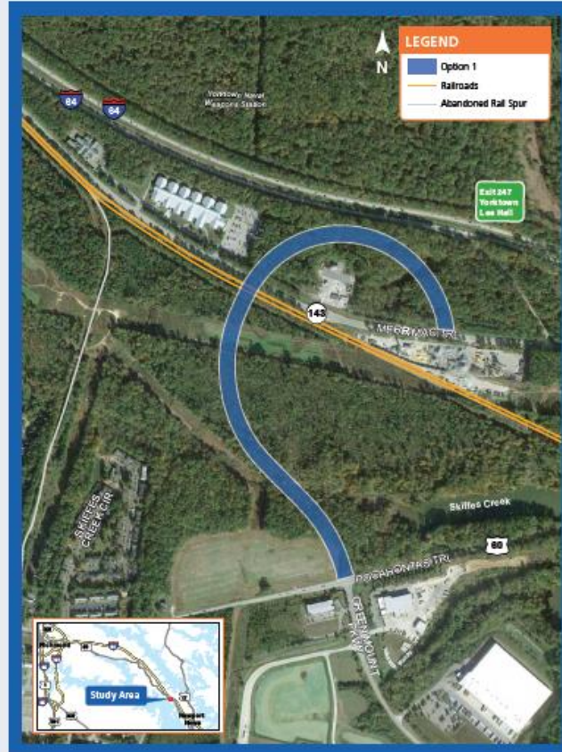
Two-lane divided facility that maintains freeway design speed (140 - foot Limit of Disturbance)
