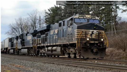
A Norfolk Southern freight train pulled by Locomotive 7565, a GE ES44DC Evolution Series diesel locomotive.
